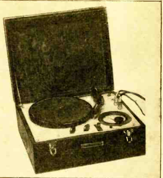
The photos herewith show the phonograph unit as designed and built by Mr. Tait, together with the crystal pickup and volume indicator. An interesting new wireless oscillator is described by the author, which permits records to be played through the receiver without direct connection. It is also possible to feed radio or microphone "pickup" into any receiver.
